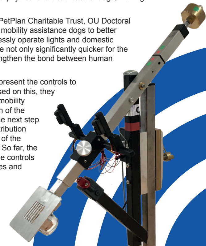
Bio-detection interface that dogs can use to signal whether disease is detected
